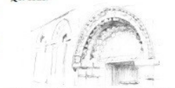
Sketch of the doorway featuring the ball and lozenge springer stone (outlined in red) and used to create the digital image
